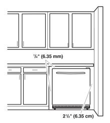
If your refrigerator is to be built-in, to ensure proper ventilation for your refrigerator, allow for  $\frac{1}{4}$ " in. (6.35 mm) space on each side and at the top. When installing your refrigerator next to a fixed wall and the hinge side is next to the wall, leave  $2\frac{1}{2}$ " (6.35 cm) minimum to allow for the door to swing open. To open door wider, leave more space.
