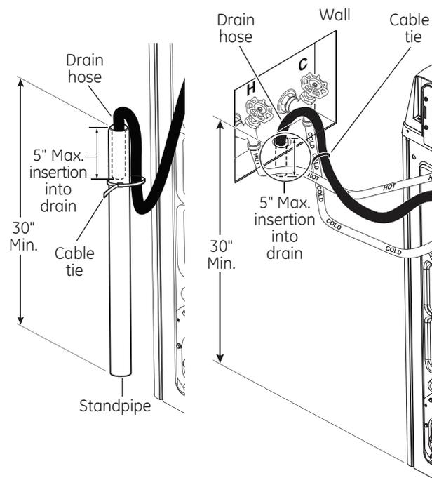
**NOTE:** Placing the drain hose too far down the drain pipe can cause a siphoning action. No more than 5" of hose should be in the drain pipe. There must be an air gap around the drain hose. A snug fit can also cause a siphoning action.
