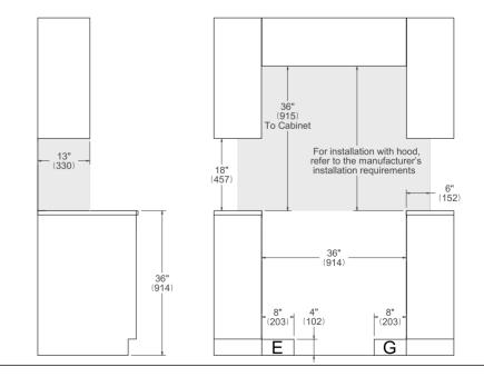
NOTE a. Electrical Connection b. Gas Connection
