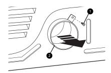
2 Press the tabs on the knockout ③ and carefully remove the knockout for the desired vent opening. (Right-side venting is not available on gas models.) Press the adapter duct ④ onto the blower housing and secure to the base of the dryer as shown.
