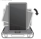
6 Using the upper groove, lift the accessory cover located at the bottom of the display. It may be tightly secured for safety. Exert some force to release it. Store the power cord in the space inside the cover. (Depending upon country)
