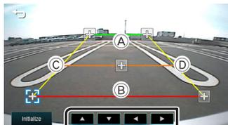
Make sure that lines A and B are horizontally parallel, and that lines C and D are of the same length.
