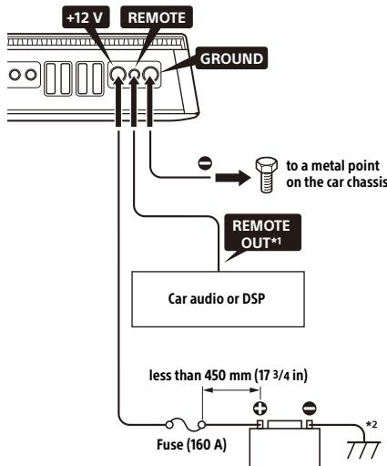
\*1 If you have the factory original or some other car audio or DSP (digital signal processor) without a remote output for the amplifier, connect the remote input (REMOTE) terminal to the ACC power supply. In high level input connection, the amplifier can also be activated without a need for REMOTE connection. However, this function is not guaranteed for all car audio or DSP.
