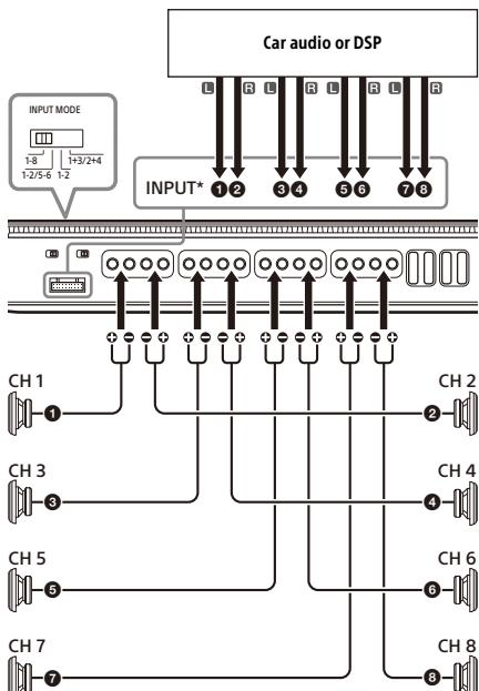
\* Connect to the INPUT/LINE OUT connector using the connection cable ③. For details, see "Input Connection" (page 11).
