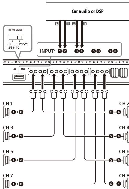
\* Connect to the INPUT/LINE OUT connector using the connection cable ③. For details, see "Input Connection" (page 11).
