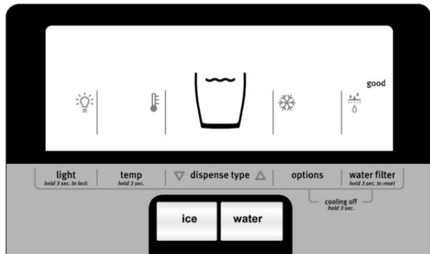
For your convenience, your refrigerator and freezer controls are preset at the factory. When you first install your refrigerator, make sure that the controls are still set to the "mid-settings." The factory-recommended set points are 37°F (3°C) for the refrigerator and 0°F (-18°C) for the freezer.
