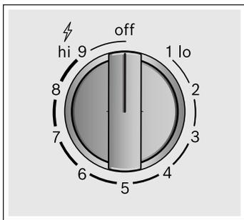
**To remove knob:** With control knob in the **OFF** position, gently lift knob up and off.
