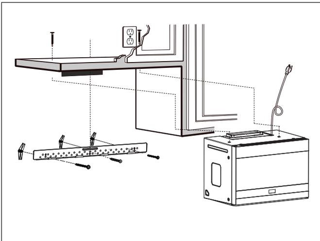
2. Place the mounting plate against the wall and insert the wing nuts into the holes in the wall to mount the plate.
