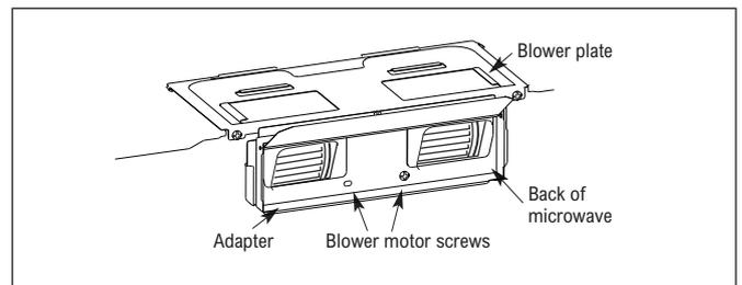
9. Secure the blower plate to the microwave with screws. Replace the blower plate in the same position.
