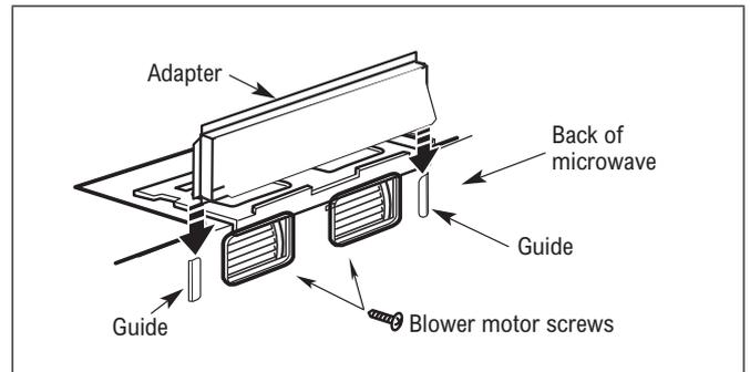
8. Secure the blower motor unit to the microwave with screws as before.
