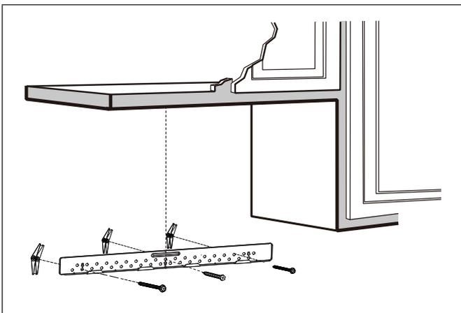
3. Tighten all bolts. Pull the mounting plate away from the wall to help tighten the bolts.
