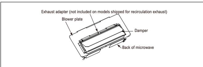
4. Attach the exhaust adapter to the blower plate by sliding it into the guides. Secure the adapter with one provided Sheet Metal Screw.
