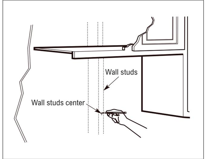
2. After locating the stud(s), find the center by probing the wall with a small nail to find the edges of the wall stud.
