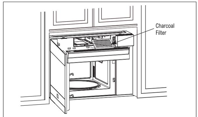
3. Install the new charcoal filter. When properly installed, the wire mesh of the filter should be visible from the front.
