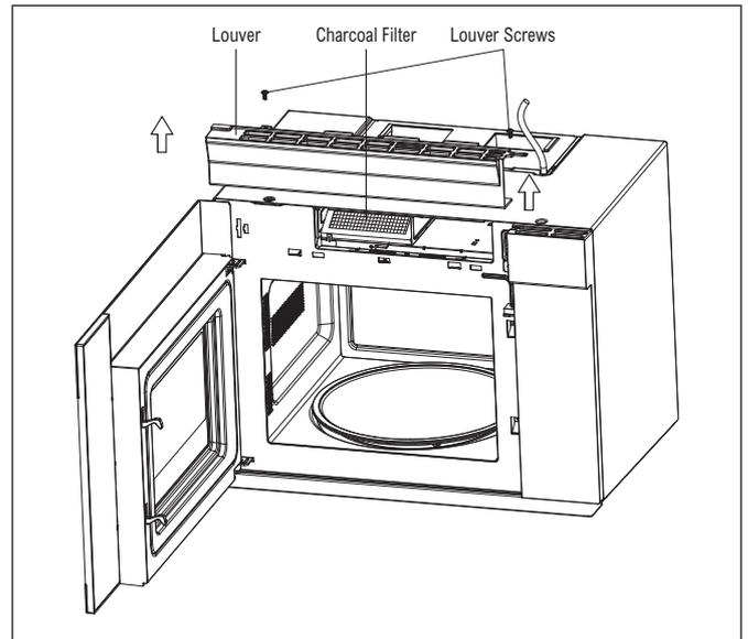
2. Open the door, remove the louver and take the used charcoal filter out.
