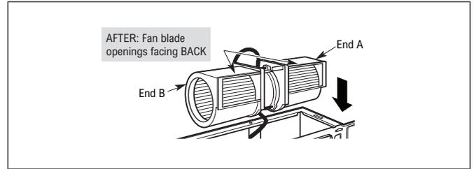
**CAUTION** Do not pull or stretch the blower unit wiring. Make sure the wires are not pinched.
