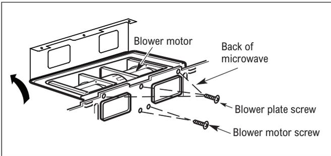
2. Carefully pull out the blower unit. The wires will extend far enough to allow you to adjust the blower unit.
