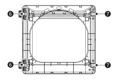
**5** With the hinges and cover caps in the new locations, remount the inner door frame onto the outer door frame with the screws removed in step 3 above.
