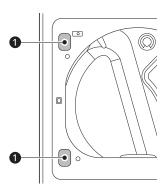
While supporting the door, remove the 2 screws on the door hinge, two from each hinge. Set the door aside face down on a protected surface to prevent damage to the door or the work surface.
