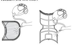
If the lint filter has become very dirty or clogged with fabric softener, wash the lint filter in warm, soapy water and allow it to dry thoroughly before reinstalling.
