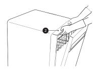
1 Align the dishwasher with the opening. Make sure the water supply line and electrical cable are in the correct positions to slide into their channels properly.
