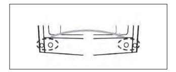
11. Place the upper door back on. Ensure the door is aligned horizontally and vertically so that the seal transfer it to the left property position. Make the middle hinge pin in the upper hole of the lower door, then tighten the bolts.
