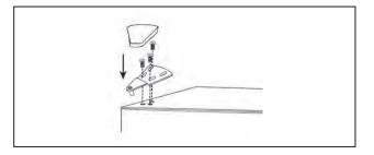
8. Transfer the lower door to the property position. Replace both adjustable feet.
