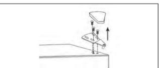
3.Unscrew the middle hinge. Lift the refrigerator door and place it in a safe place to protect it from damage and scratches.
