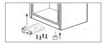
10. Make the middle hinge reverse the direction 180°, then transfer it to the left property position. Make the middle hinge pin in the upper hole of the lower door, then tighten the bolts.
