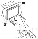
2 When the lower level is removed, remove from the upper two catches of the trim plate (5).
