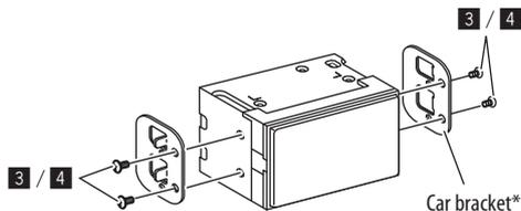
**Note:** Select the appropriate screws (supplied) for the mounting bracket.
