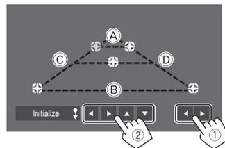
Make sure that **A** and **B** are horizontally parallel, and that **C** and **D** are the same length.
