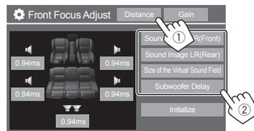
[Sound Image LR (Front)] Locates the sound image in front of the front seats, and adjust the balance.
