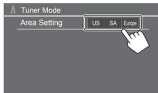
**[US]** (initial) Select this when using this unit in North/Central/South America. FM and AM intervals are set to 200 kHz and 10 kHz respectively.
