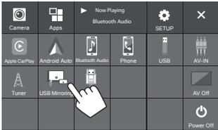
The Android device screen is displayed on the monitor screen of this unit. You can access your Android device from this unit.
