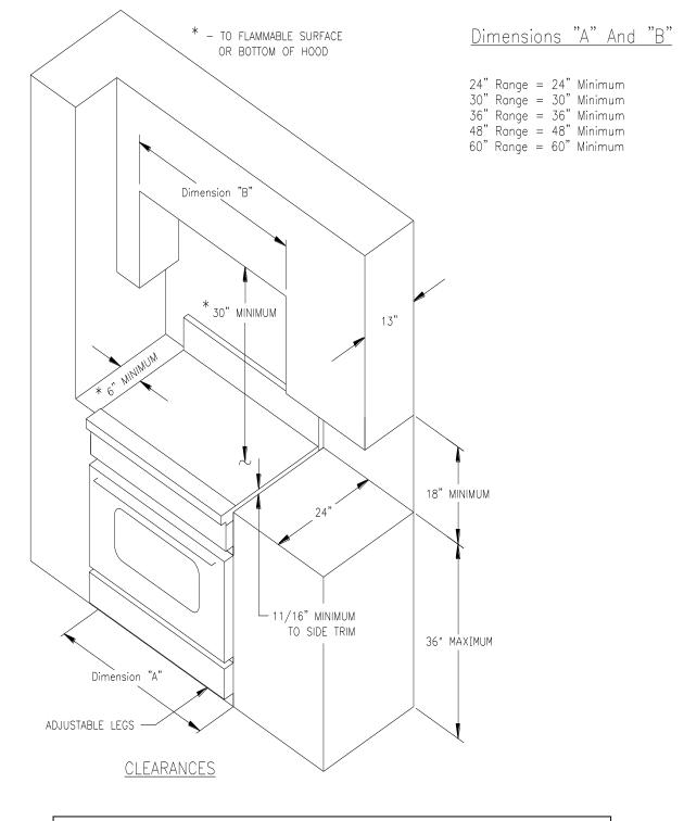
The maximum depth of cabinets installed above cooling tops be 13"
