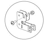
Clamp the lower brackets together using the supplied M6 screw and Nut. Secure using a 3/16" (4mm) Allen key and 3/8" (10mm) spanner. Ensure brackets are clamped tightly before proceeding.
