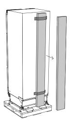
Remove the trims kit from the back of the appliance. Refer to 'Supplied parts' - Trims install kit for parts included in the box.
