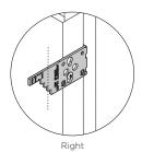
Check if the gaps between appliance and cabinetry side walls are even on left and right sides.
