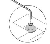
Loosen the M8 screws by 1/8" (3mm).
