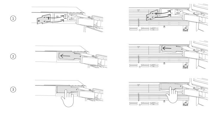
Place the hinge pocket cover to the hinge pocket, matching the studs on the cover to the slots in the hinge pocket.
