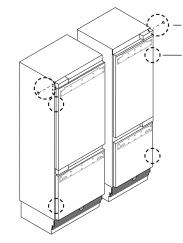
Insert the barbed plugs into large holes on the top right and left sides of both appliances.
