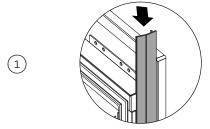
Insert door side covers into the gaps on the right and left sides of the drawer and slide downwards to clip into place. Press firmly to secure.
