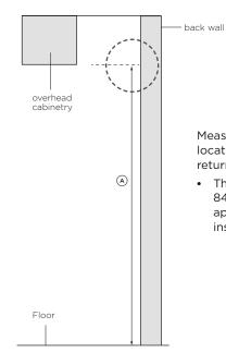
Measure the height (A) of the attachment location from the floor to the alcove return.
