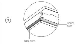
Attach the peeled portion starting from one end of flange perpendicular to top end of long trim.
