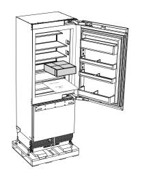
Remove the installation kit and miscellaneous items kit from inside the appliance.
