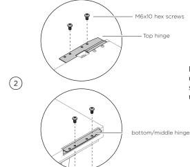
Detach the door from the appliance by unscrewing the door hinge M6x10 hex screws (4x) at the top hinge and bottom/middle hinge.
