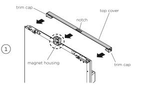
Align the top cover to the top of the door. Clip the notch into the magnet housing, and the trim caps on top of the adhesive strips.
