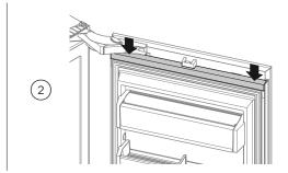
Press down both ends of the top cover to engage the trim caps on the adhesive strips.
