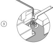
Screw the M8 washer and nut to the adjustment screw and loosely tighten.
