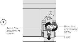
Turn the front and rear adjustment screws clockwise to raise height of the appliances and counter-clockwise to lower the height.
