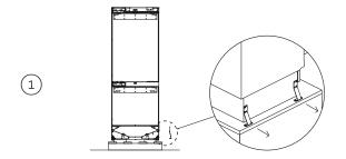
Remove the brackets from the non-hinge side of the pallet.
