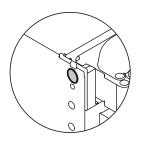
Before rolling into the cavity, insert a barbed plug into the large holes at the top right and left sides of the appliance.
