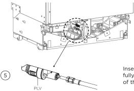
Insert the tube end of the adaptor fully into the PLV at the bottom front of the appliance.
