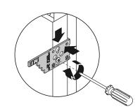
Loosen the right and left screws at the top and bottom sides of the door.
