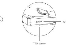
Release the hinge spring by turning the T20 screw in the hinge to the '0' position. Close the door and lay the appliance on its back on the pallet.
