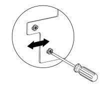
To adjust the door panel further, loosen the M8 washer and nut and slide the door panel to suit. If further adjustment is still required, remove the door panel then loosen the fixing screws of the hanging bracket and move bracket sideways to suit.
