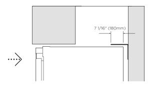
Roll the appliance carefully into the cabinetry until the anti-tip bracket overlaps the back edge of the appliance.
