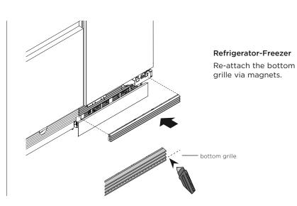
For toe kick heights 4 1/2" - 5" (114 - 127mm), shorten the bottom grille by cutting along the vertical ribs.
