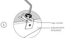
Loosen the cap screws of the adjustment brackets on both sides of the plinth with a hex key.
