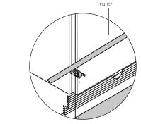
Check the alignment gauges while adjusting the screws to maintain the alignment of the appliance.
