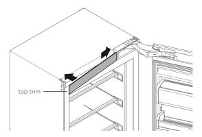
Slide one end of the top trim into the hinge pocket of the appliance.
