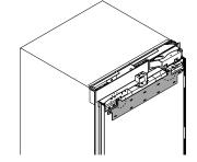
Remove the M8 nut and M8 washer from the M8 screw at the top of the door using the supplied hex key and spanner.
