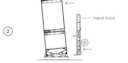
Tilt the appliance slightly forward and insert the hand truck between pallet and appliance.
