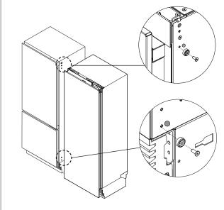
Remove bolts from the locations marked via the green labels on your appliance. Add the flange joiners, and tighten using a 1/8" (3mm) Allen key to secure.
