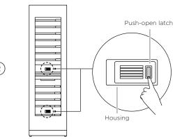
Open the cover of filter housing by pushing the latch.
