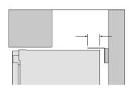
If minimum 7 1/16" (180mm) overlap cannot be achieved, install a solid spacer to the wall stud behind the bracket.
