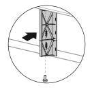
Press the flow divider firmly against the bottom of the door/drawer panel. Ensure the adhesive layer side of the divider contacts the door panel. Secure the air flow divider to the panel with screw.
