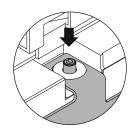
Hold the door panel at an angle from the top of the door and lower the screw holes of the hanging bracket onto the adjustment screws. .
