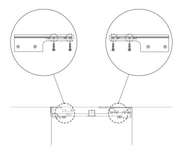
Fix the top brackets to the ceiling surface of the cabinetry with 8Gx16 countersunk screws.
