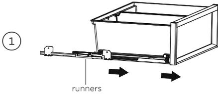
To remove a bin, extend the bin on its runners, and empty the bin.
