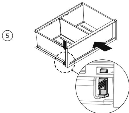
Push the bin slowly onto the securing tabs until you feel it clip onto the runners. Ensure the bin tabs are clipped securely onto the runners before use.
