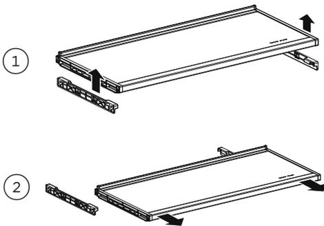
To remove, hold the front and back edge of the shelf firmly.
