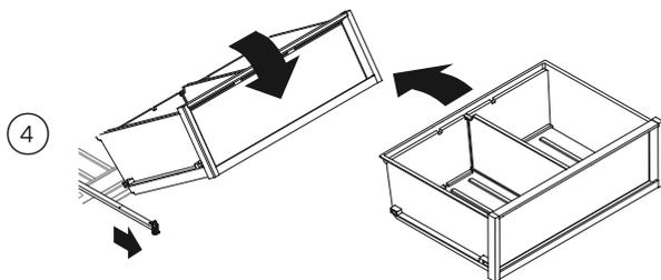
To return the bin, extend the runners and place the bin on top of the runners.
