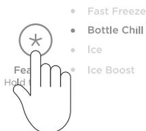
When activated, an alarm will sound, **BOTTLE CHILL** will flash and
