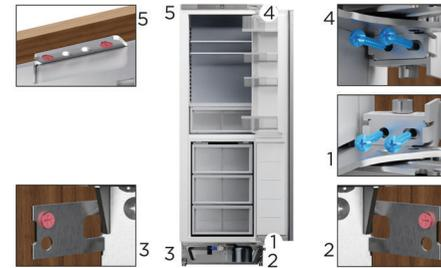
Open the door and secure following the sequence shown. The longer screws should be used where shown in blue, and the smaller screws where shown in red. Ensure a gap between drill and product is maintained to avoid cosmetic damage.
