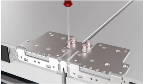
Secure the bracket at the front top using four screws.
