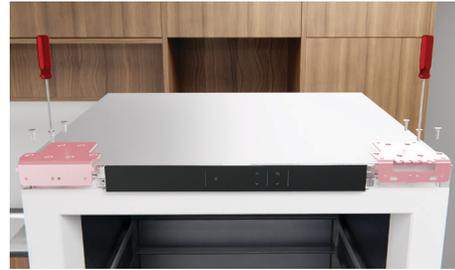
Swap alcove bracket with the hinge bracket. Secure using 3 screws at the top of the cabinet.
