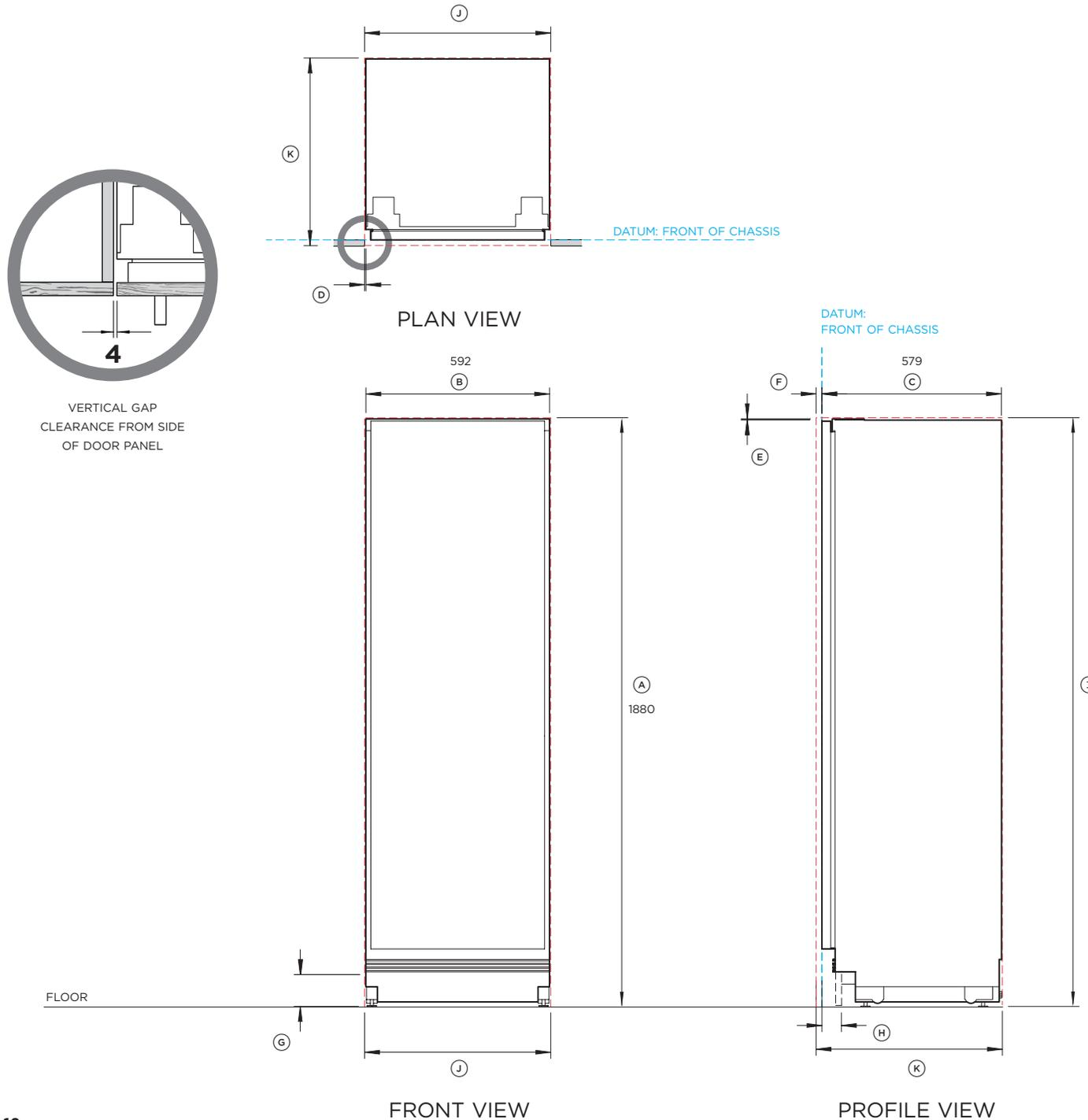
NOTE: Left hand hinge is a mirrored version of the image shown. Left hand hinge can be achieved using supplied parts.
