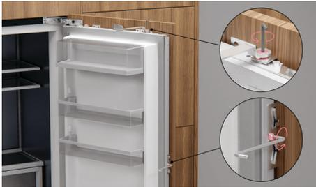
Remove the flow divider and panel bracket before removing all door panel side screws and the M8 washer and nut. Lift panel up and out to remove.
