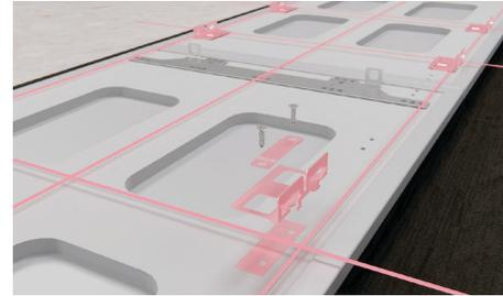
Remove all blue tape from the panel. Align side brackets to the pre-drilled holes based on your hinge orientation. Red labels indicate left hinge installations, blue labels indicate right hinge installations.
