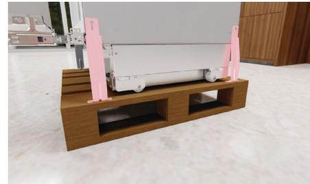
Using a Phillips screwdriver, unscrew the transit brackets from one side of the product and set aside.
