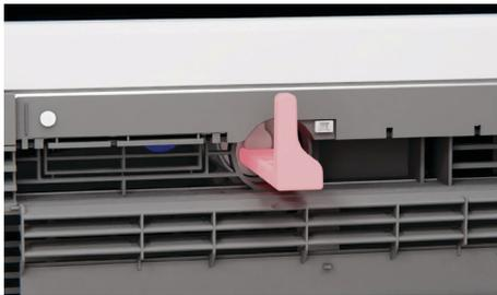
Using the filter tool, rotate filter 90° anti-clockwise to unlock and remove.
