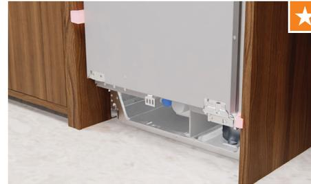
Push product into alcove. Push in until the gauges touch the alcove end. Ensure hose doesn't bend or kink and that the power cord is not trapped.
