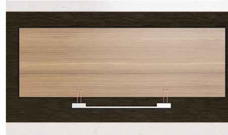
Ensure all bracket and handle holes have been pre-drilled. Refer to 'custom panel preparation' for details.
