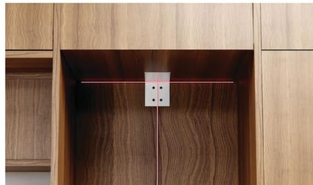
Measure the height from floor to the front overhang and mark on rear wall.
