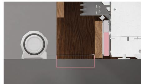
Push the toe kick back to the desired depth before removing. If toe kick depth is less than 3 9/16" (90mm), attach the additional foam block.
