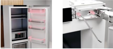
Open the door and remove the door shelves. Loosen the hinge screws using the supplied Torx T25 driver. Slide the door out and place onto a protected surface.
