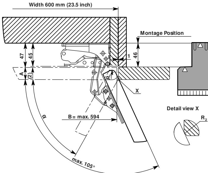
Cabinet frame wall thickness 16 mm
