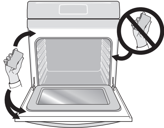
Figure 22: Clean around the oven door gasket
