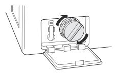
Close the drain pump filter cover.
