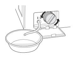
Clean the pump filter and opening.
