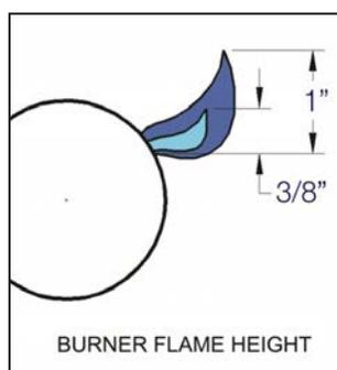
Flames should be blue and stable with no yellow tips (LP units will have some yellow tipping). There should be no excessive noise or flame lifting. If any of these conditions exist, remove the burners and check if dirt, debris, spider webs, etc., are blocking the air shutter or burner ports. Proceed with air shutter adjustment if necessary.
