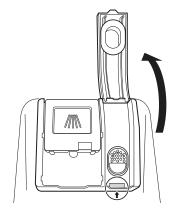
Add a liquid rinse aid to the maximum fill level. Allow the rinse aid to settle in the dispenser while filling, or air bubbles may result in poor drying performance. Avoid overfilling the dispenser.
