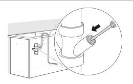
**2** Attach the drain hose to the waste tee with the hose clamp provided. Move the clamp into position and tighten it with a flat-blade screwdriver.
