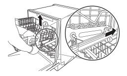
To replace the rack, place the back rack supports behind the rear hooks and pull the rack forward to snap the supports into the hooks. Then align the front rack supports with the front hooks and push the front of the rack down to snap the supports into the front hooks.
