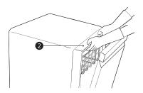
Align the dishwasher with the opening. Make sure the water supply line and electrical cable are in the correct positions to slide into their channels properly.
