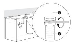
**3** If it is not connected, attach the rubber hose connector to the disposal or waste tee with a hose clamp (not provided).
