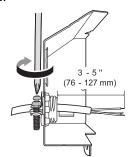
7 Pull the existing wires through the openings in the junction box. Tighten 2 screws 4 to reassemble the junction box in the appliance.
