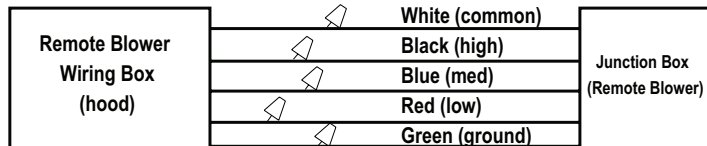
CBE-1000 / PBN-1000A: WIRING DIAGRAM
