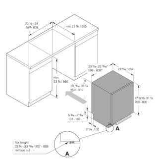
$\mbox{\ensuremath{\,\star}}$  Flexible side trims (width without side trims: 23  $\ensuremath{\,\%_{16}}$  / 596)
