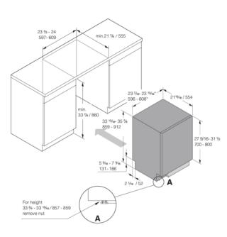
$\mbox{\ensuremath{\mbox{\$}}}$  Flexible side trims (width without side trims: 23  $\%\mbox{\ensuremath{\mbox{\$}}}_{6}$  / 596)
