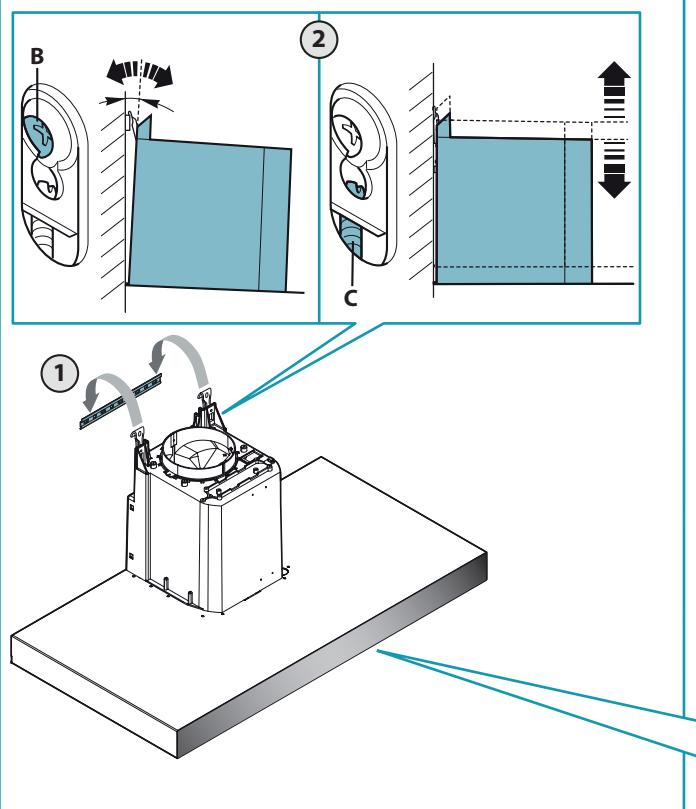
EN - Hood fastening (1), check valve installation and suction pipe assembly (3).
