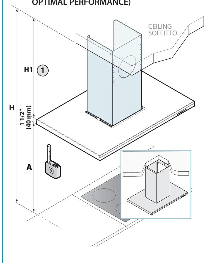
EN - Installation on ceiling with/without false ceiling
