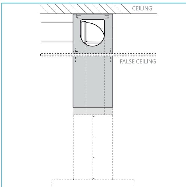
**EN** - Side outlet which can only be used with false ceiling.
