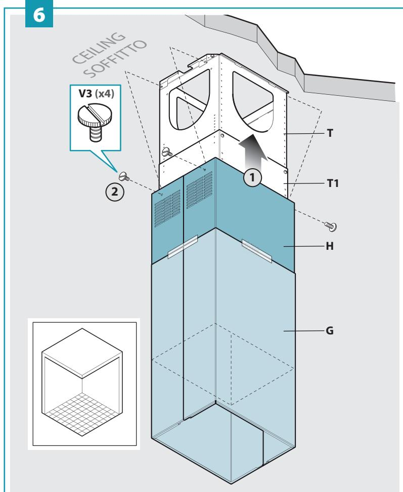
EN - INSTALLATION ON CEILING with false ceiling
