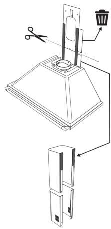
5. Insert the inner sliding chimney into its base.
