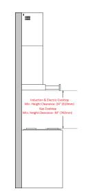
For optimal performance, the distance from the cooking surface to the bottom of the range hood should be between 24" and 30", unless otherwise noted. DO NOT install a range hood less than 24" above cooking surface.
