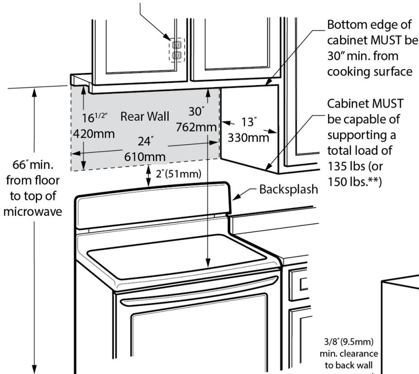
\*When installing beneath smooth, flat cabinets, refer to cabinet template for detail power cord clearance instructions.
