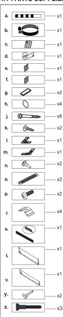
The parts required for positioning the dishwasher are in plastic bags. Check that all of the following parts are contained in plastic bags.
