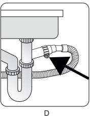
Use hose clamp that shown at the Figure 4. for drain hose assembly to the sink.
