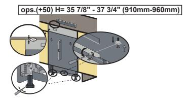
If the height of the enclosure is above 35 7/8" (910mm) use long supports as shown in the figure.
