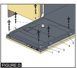
7- As shown in Figure D, Screws Ø 5/32" x 53/32" (Ø 4mm x 42,5mm) is installed in positions I,III and V.
