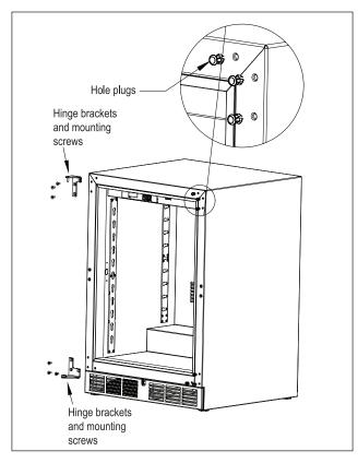
Figure 8. Hinge Removal
