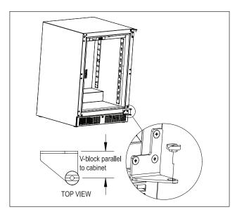
Figure 15. Installing V-Block
