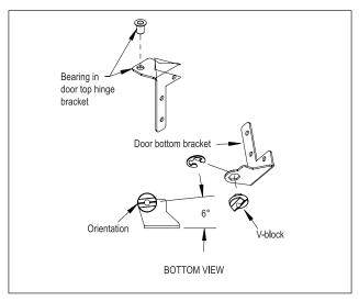
Figure 13. Bearing and V-Block
