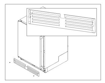
Figure 5. Toe Kick Installation
