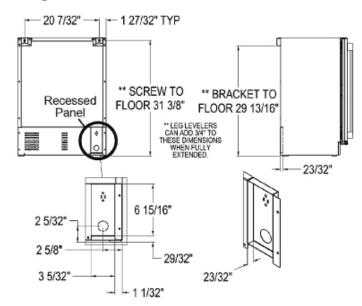
Figure 1. HH (Sottile Model) Electrical Connections
