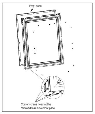
Figure 11. Removing Front Panel
