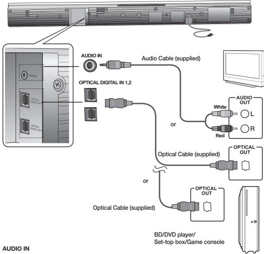
Connect AUDIO IN on the main unit to the AUDIO OUT of the TV. Be sure to match connector colors.
