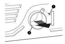
Press the adapter duct 3 onto the blower housing and secure it to the base of the dryer as shown.
