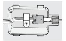
4. Reattach the electrical harness by positioning the cable clips over the black markings on the harness and push the 4 cable clips through the openings in the rail to secure the harness in place.
