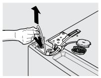
Use care while pulling the water tube from the door to be sure the tube does not kink.
