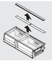
Removing Auto Humidity Control Membrane
