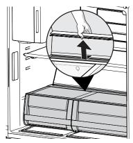
Removing Auto Humidity Control Membrane
